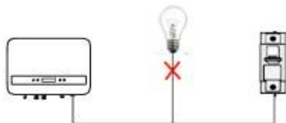
Incorrect Connection between Load and Inverter
